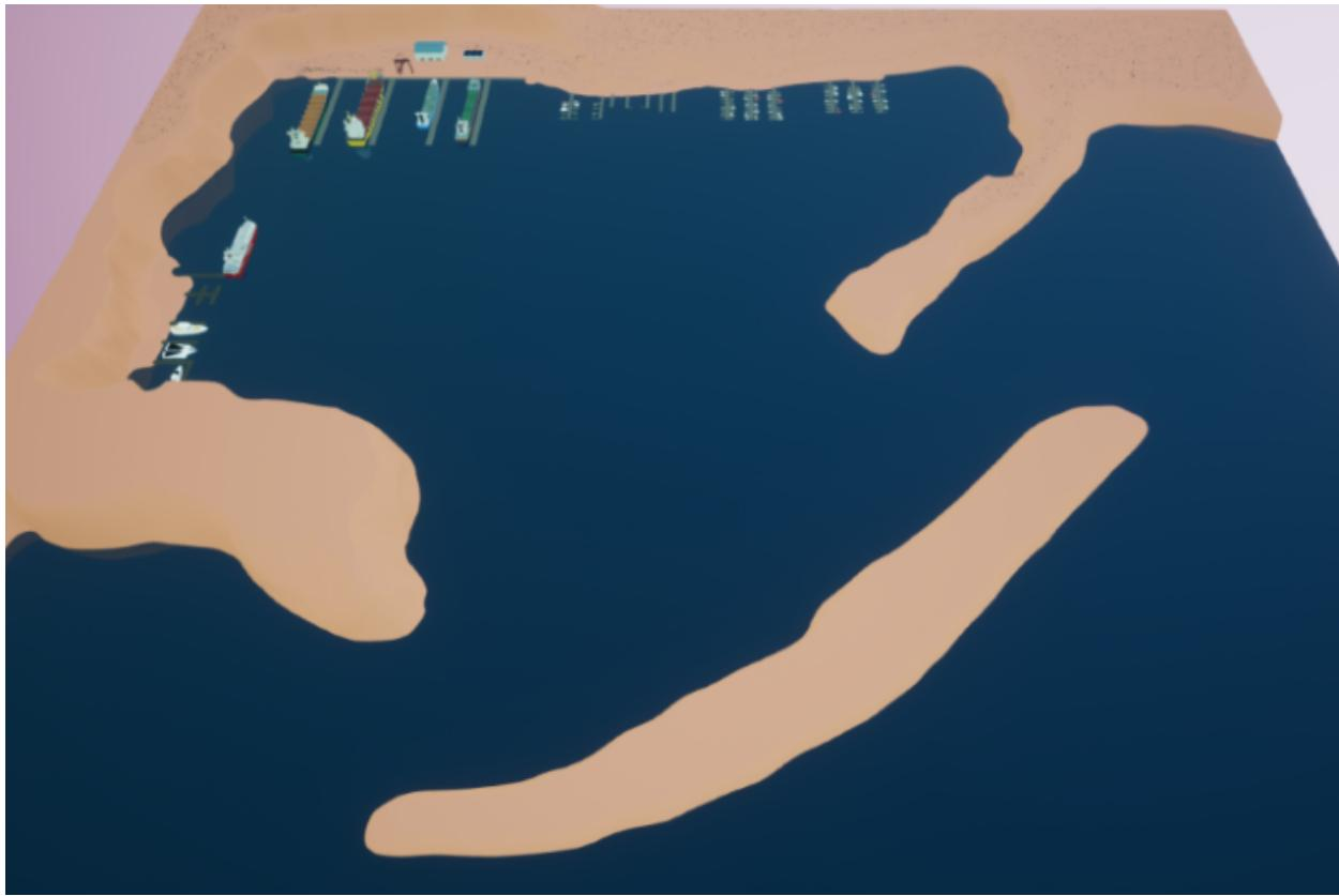
This environment has a number of different sized piers that can be inspected. Total environment size is about 2km x 2km. There are 3 sizes of piers ranging from small fishing docks to larger freight sizes, which boats included.
